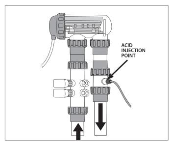
Figure 3. Chlorinator Cell and Doser Installation
