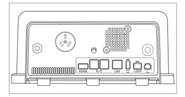
Figure 8. Halo Chlor Connections
