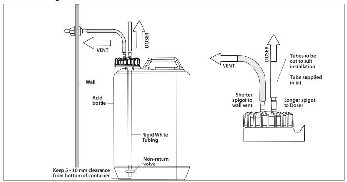
Figure 5. Vent Kit Installation Diagram
