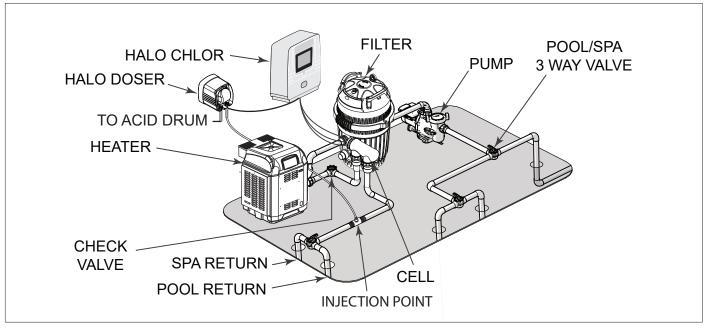
Figure 2. Typical Installation Diagram
