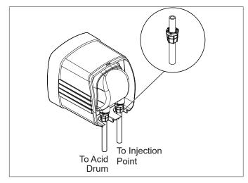
Figure 6. Halo Doser Tubing Connections
