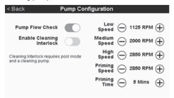
Figure 30. Halo Pump Configuration Flow Check Screen
