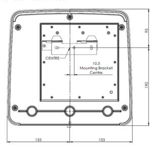
Figure 4. Mounting dimensions
