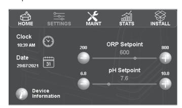
Figure 36. Halo ORP and pH Setpoint Screen
