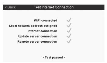
Figure 38. Halo Test Internet Connection Status Screen -WiFi
