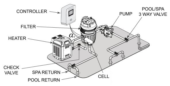
Figure 3. Typical Installation Diagram
