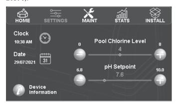
Figure 35. Halo Pool Chlorine and pH Setpoint Screen
