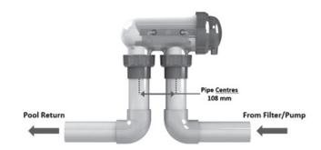
Figure 5. Chlorinator Cell Installation
