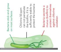
Bacteria cling to surfaces (walls, floor, piping systems and especially in the filter media)
