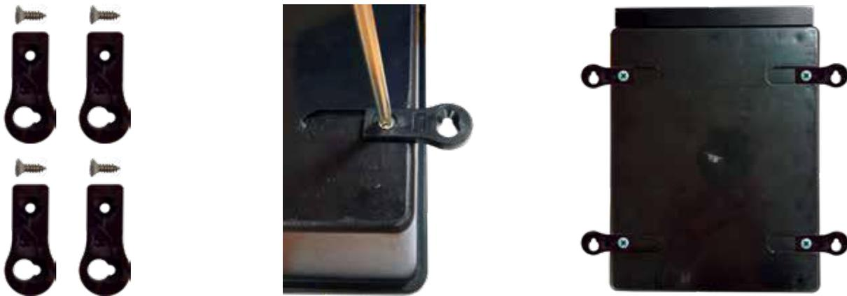
**IMPORTANT:** ONLY use a hand screwdriver to fasten the mounting lugs to the enclosure until the screws are firm. Use of a power tool will strip the threads out of the plastic.
